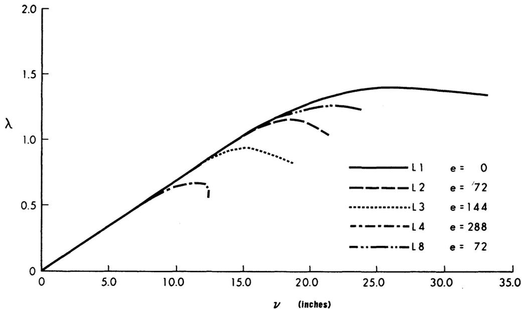
Fig. 7. Load-displacement response structures L 1-L 4, L 8.
