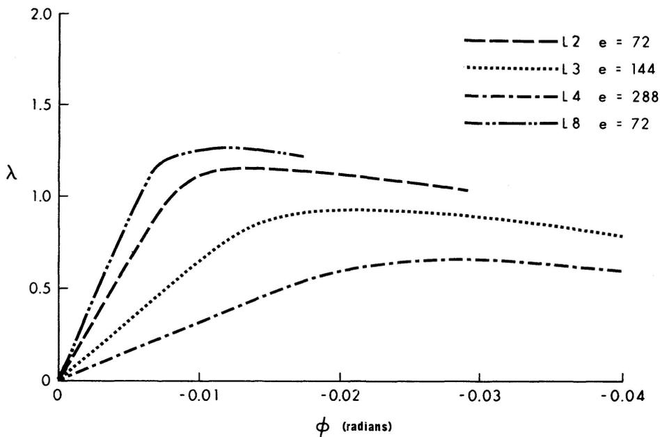
Fig. 8. Load-floor rotation response structures L 2-L 4, L 8.
