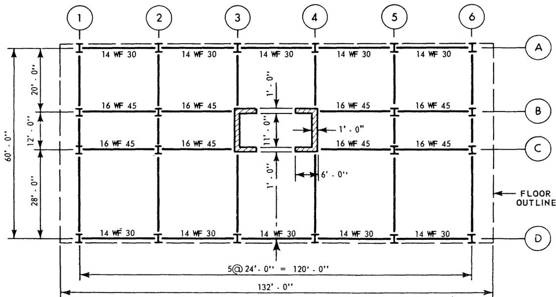
Fig. 5. Plan twenty-four story structure L.
