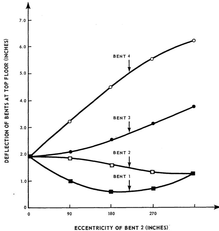
Fig. 3. Bent deflections at top floor.
