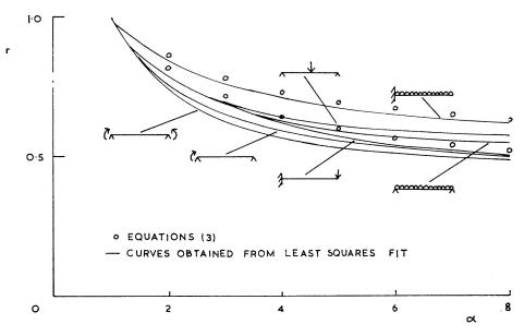
Fig. 10. Effect of loading and support conditions on reduction curve.
