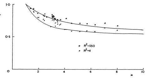
Fig. 9. Comparison of reduction formulae with numerical results for arbitrarily tapered cantilevers – uniform load.
