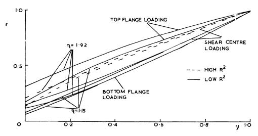
Fig. 5. Reductions in stability caused by linear flange breadth curtailment.
