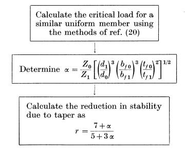
Fig. 11. Procedure for estimating the critical load for a tapered beam.
