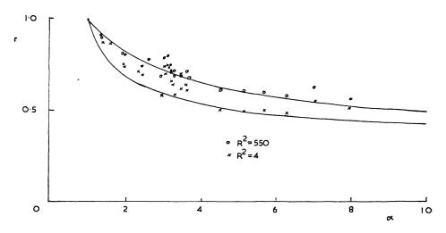
Fig. 8. Comparison of reduction formulae with numerical results for arbitrarily tapered cantilevers – end load.
