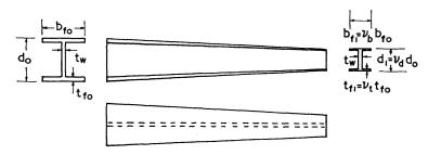
Fig. 1. Tapered I-section.
