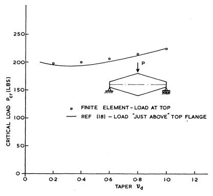
Fig. 3. Comparison of results for depth tapered section.
