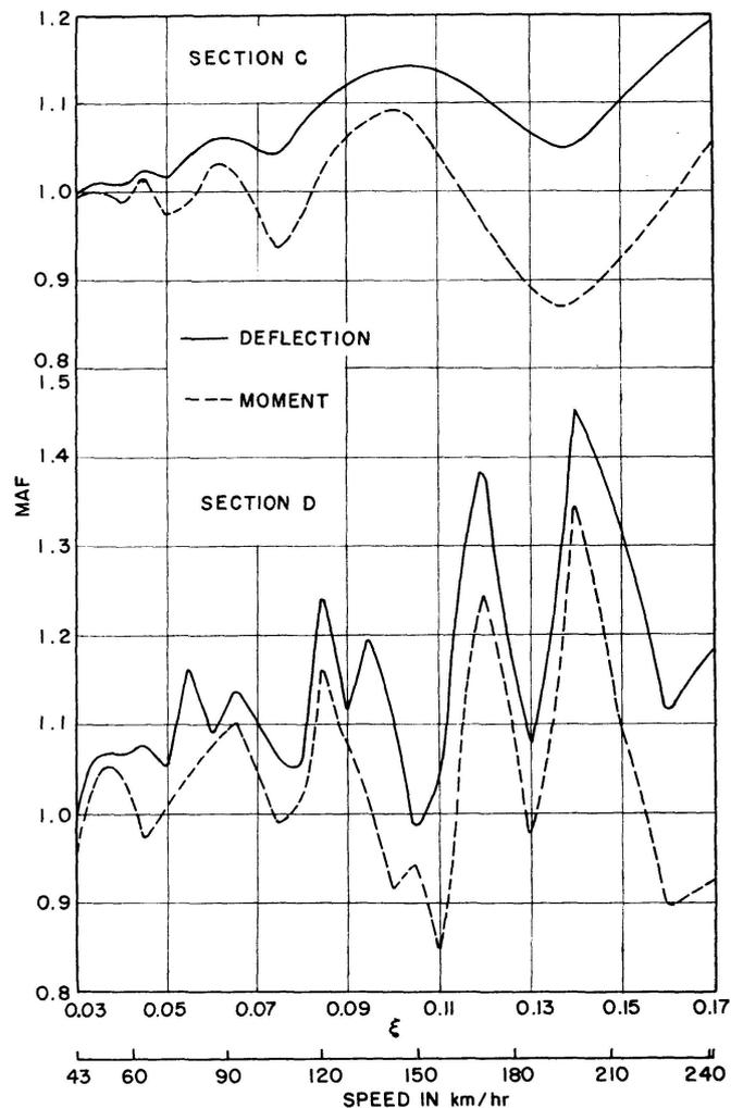
Fig. 6. Amplification spectra for the cantilever bridge III, sections C and D.
