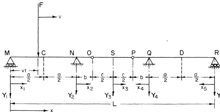
Fig. 1. Cantilever bridge under moving force.
