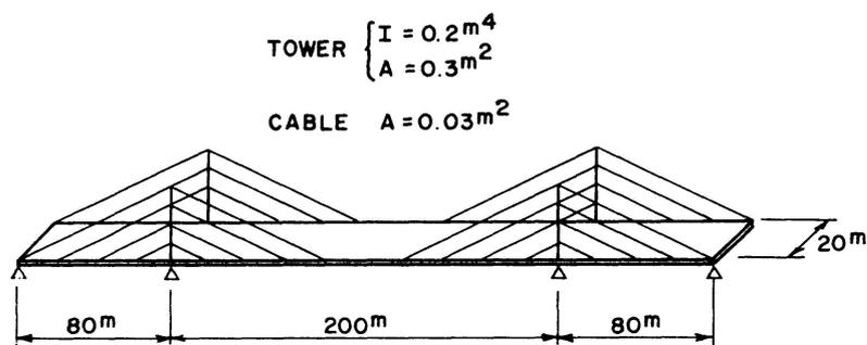
Fig. 6. Example bridge for dynamic analysis.
