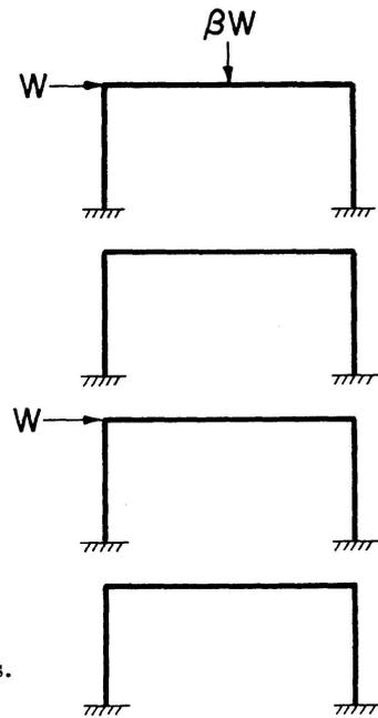
Fig. 4. One Cycle of Load Applications.
