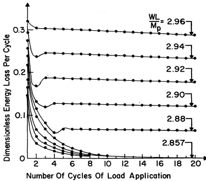
Fig. 12. Energy Loss per Cycle Versus Number of Cycles of Load Application.
