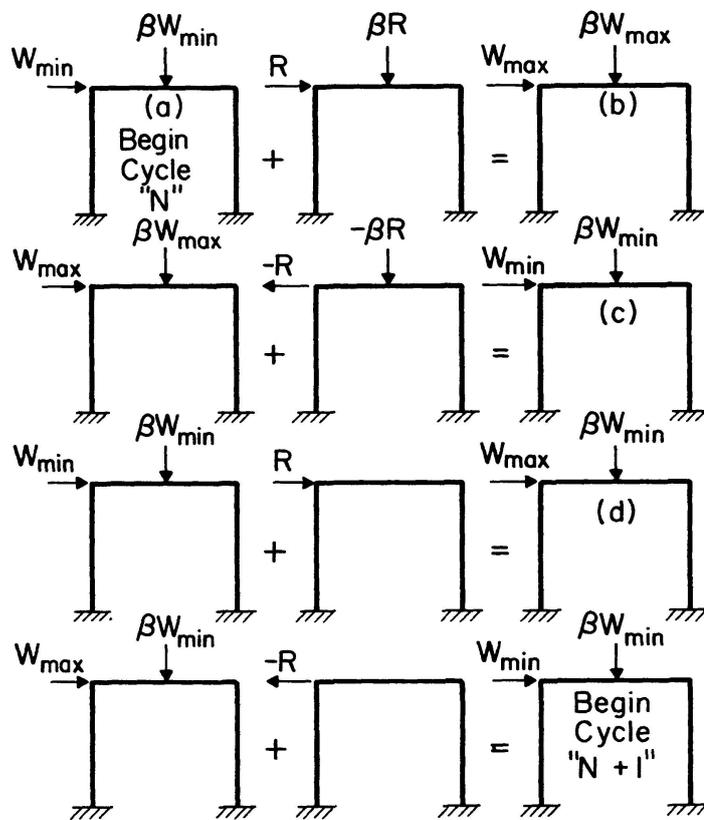
Fig. 7. The  $N$ th Cycle of Load Applications.
