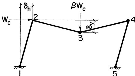
Fig. 6. Collapse Mechanism.
