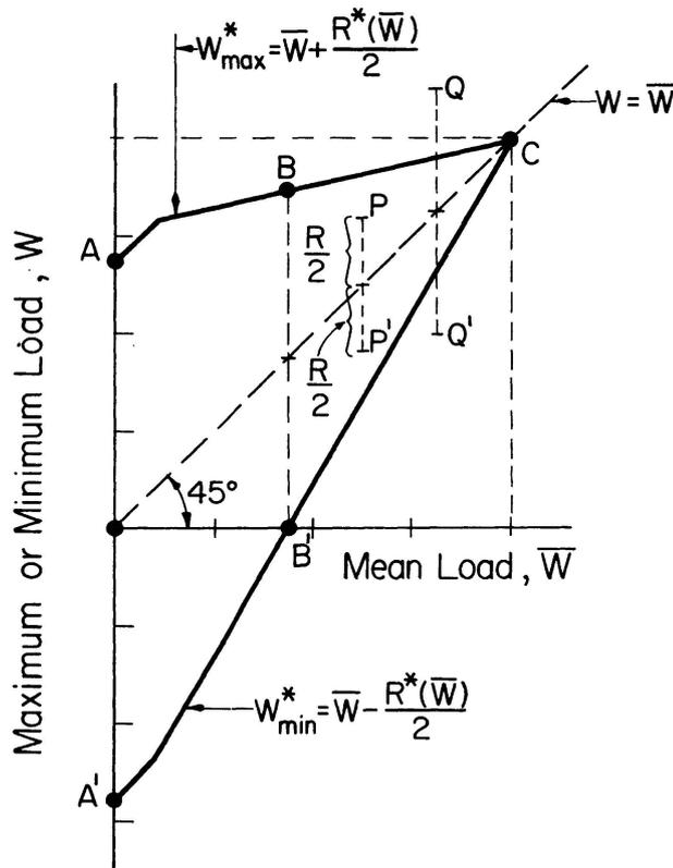
Fig. 2. Maximum or Minimum Load Versus Mean Load.
