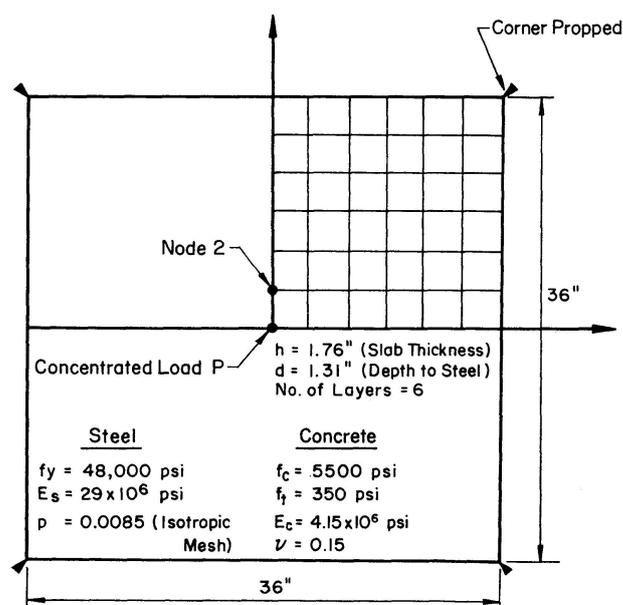
Fig. 5. Material properties and finite element mesh for corner-propped slab.
