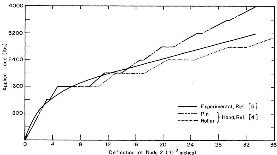
Fig. 7. Effect of inplane boundary conditions on computed deflections of corner-propped slab (after HAND, ref. [4]).
