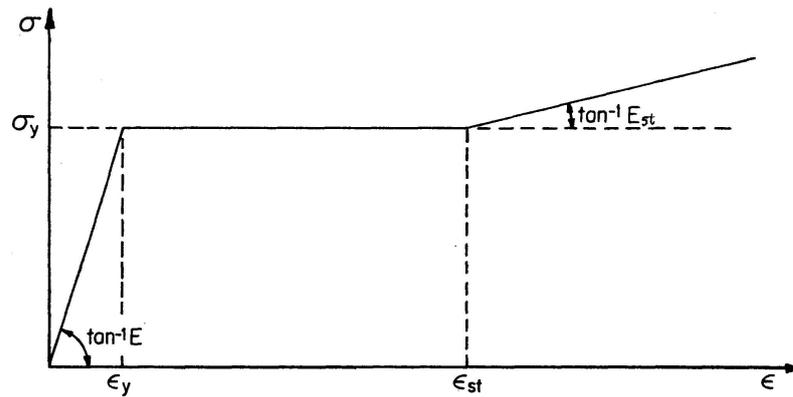
Fig. 2. Idealized stress-strain diagram (in tension and compression).
