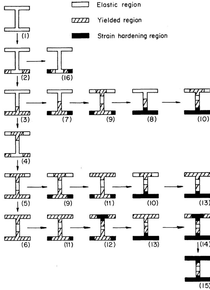
Fig. 4. Sequence for checking the strain patterns.
