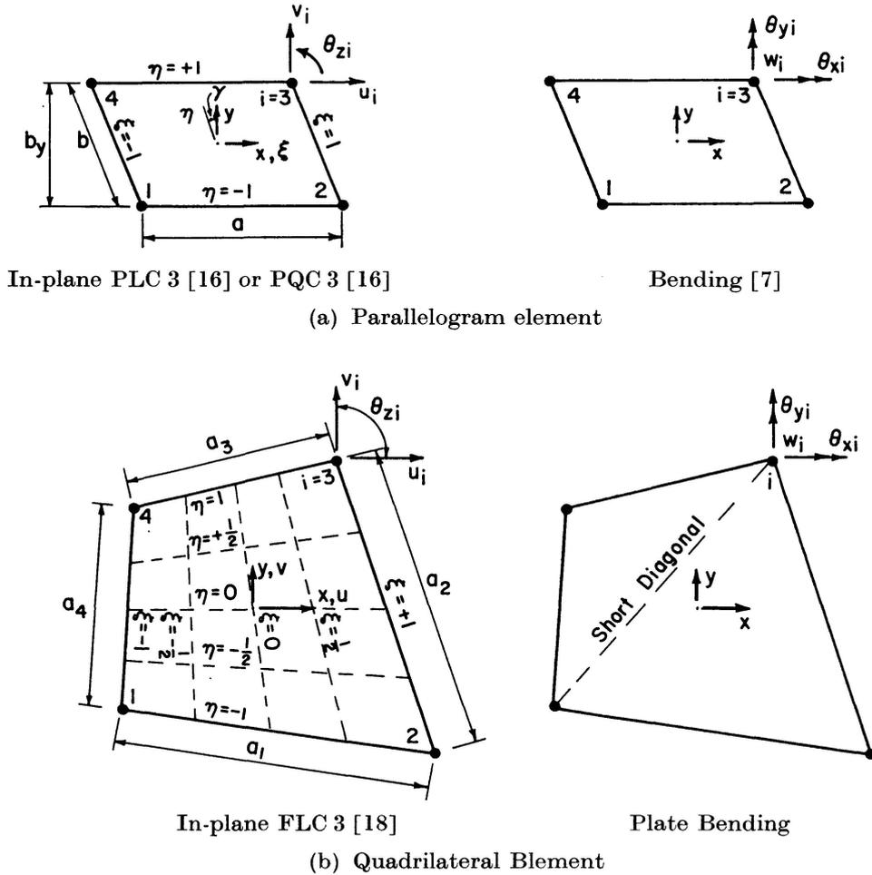
Fig. 6. Elements for complex box girder bridges.
