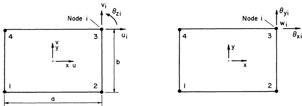
(a) Abu Ghazaleh's in-plane element [1]      (b) Rectangular plate bending element [22]
