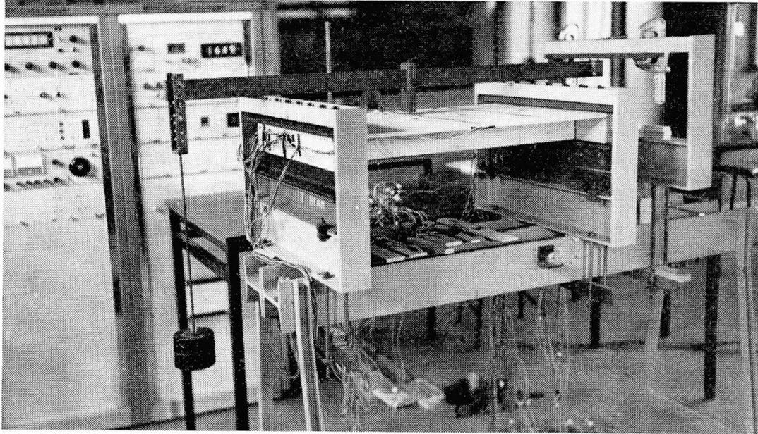
Fig. 3. Model test set-up and the data logger.
