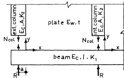
Fig. 15. Load acting at frame joint.
