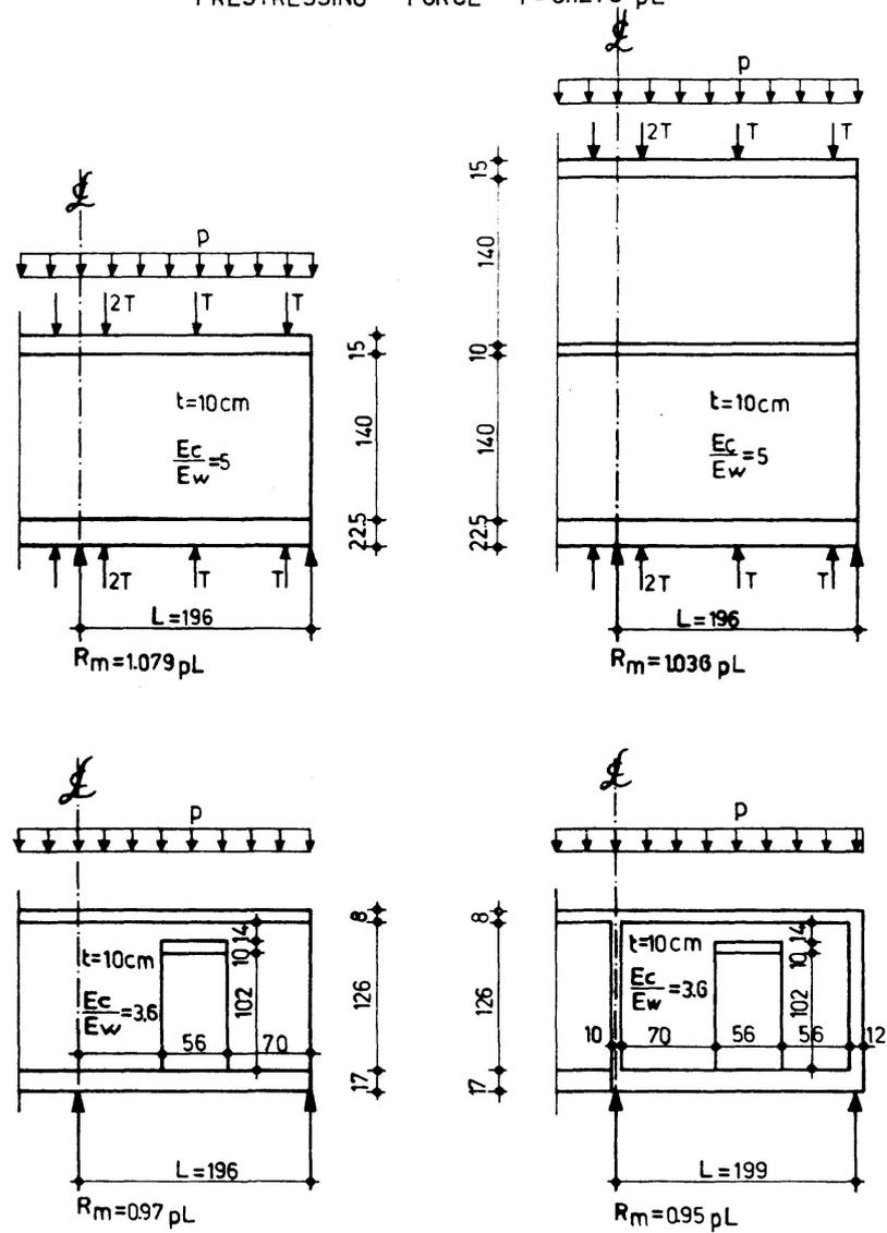
Fig. 16. Redundant reactions of continuous composite walls.
