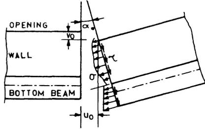
Fig. 5. Displacement components of edges.
