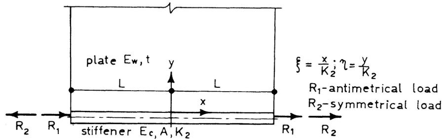
Fig. 13. Load acting in line with stiffener axis.
