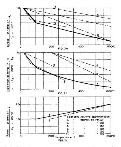
Fig. 2. Effect of temperature on concrete stress-strain properties.
