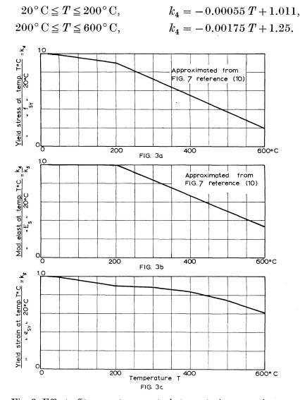
Fig. 3. Effect of temperature on steel stress-strain properties.
