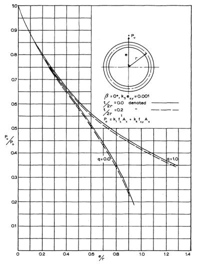
Fig. 6. Comparison of wall thickness ratio t/2r variation.
