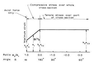
Fig. 5. Limiting values of maximum compressive strain at ultimate load.
