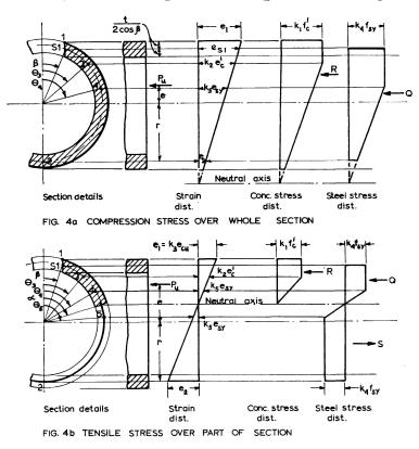
Fig. 4. Stress and strain distributions at ultimate load.
