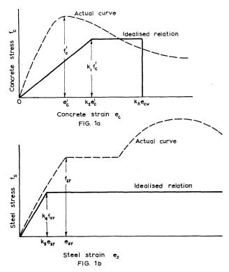
Fig. 1. Stress strain properties of concrete and steel.
