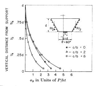
Fig. 11. Stress Distribution of  $\sigma_y$  at Critical Section.
