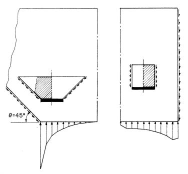
Fig. 5. Distribution of the Reaction Forces for a Continuous Supporting Pad (c=b).
