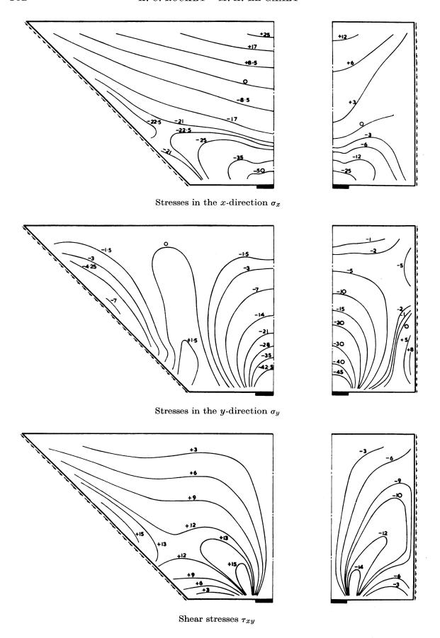
Fig. 8. Stresses  $\sigma_x$ ,  $\sigma_y$  and  $\tau_{xy}$  (Ksi).
