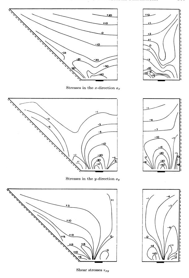
Fig. 7. Stresses  $\sigma_x,\,\sigma_y$  and  $\tau_{xy}$  (Ksi).
