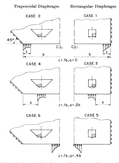
Fig. 3. Variation of the Distribution of the Reaction Forces with a Change in the Position of the Bearings, the Width of all the Bearings Being Constant (= 0.1b) Diaphragms, b/d = 1.
