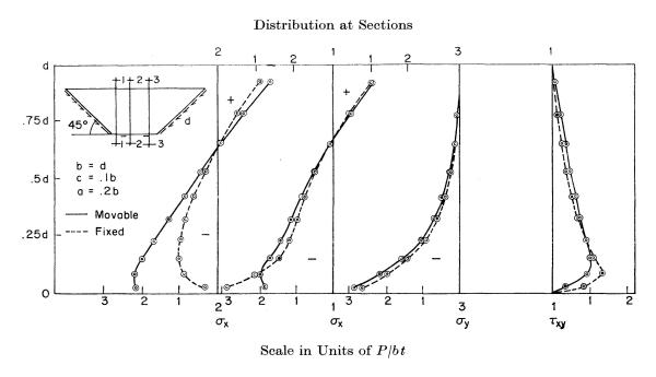
Fig. 13. The Effect of Preventing any Horizontal Movement Along the Length of the Supporting Pad on the  $\sigma_x$ ,  $\sigma_y$  and  $\tau_{xy}$  Stress Distributions.
