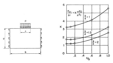
Fig. 14. Buckling Load Coefficient for Rectangular Web Plates Subjected to In-Plane Patch Loading (Reference 11).
