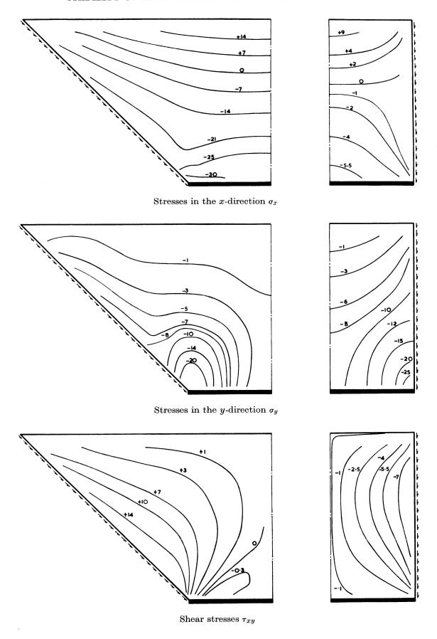
Fig. 9. Stresses  $\sigma_x$ ,  $\sigma_y$  and  $\tau_{xy}$  (Ksi).
