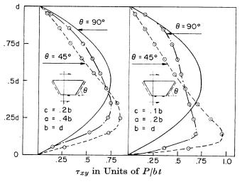
Fig. 12. Shear Stress Distribution Across the Depth.
