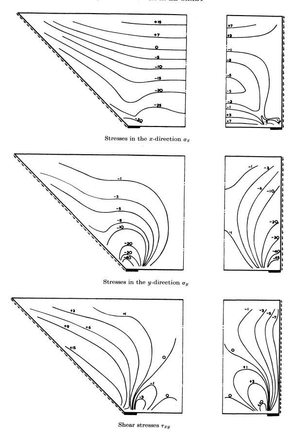
Fig. 6. Stresses  $\sigma_x$ ,  $\sigma_y$  and  $\tau_{xy}$  (Ksi).
