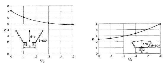
Fig. 17. Buckling Load Coefficient for Various c/b Values (b = d,  $\theta = 60^{\circ}$ ).
