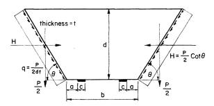
Fig. 2. Dimensions of a Typical Diaphragm.
