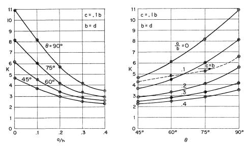
Fig. 15. Buckling Load Coefficient for Various a/b and  $\theta$  Values (b=d, c=0.1b).
