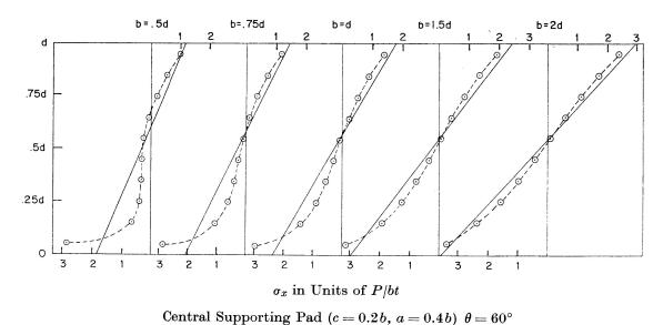
Fig. 10. Stresses  $\sigma_x$  Across the Depth at the Edge of the Supporting Pad – Comparison with Elementary Beam Theory.
