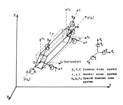
Fig. 1. Coordinate Axes System and Member Freedoms.
