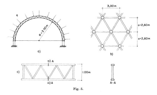
It is a dome of 300 m in diameter, whose members are steel trusses with 1 m depth.
