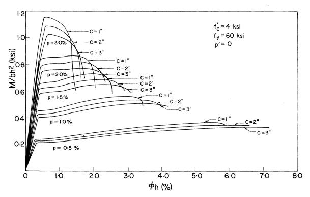
Fig. 18. Effect of concrete cover on ductility:  $M-\phi$  diagrams.
