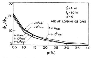
Fig. 21. Effect of loading duration on ductility:  $\phi_u/\phi_y$ -p diagrams.
