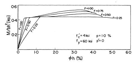
Fig. 8. Effect of bond on ductility:  $M-\phi$  diagrams.
