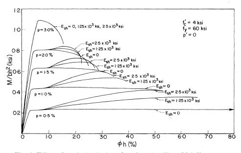
Fig. 6. Effect of strain-hardening of steel on ductility: M- $\phi$  diagrams.
