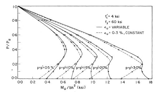
Fig. 24. Interaction diagrams for symmetrically reinforced sections.
