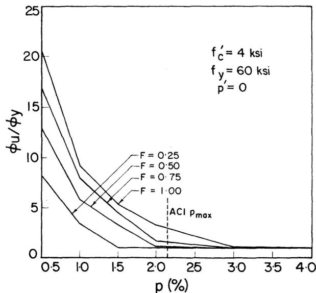
Fig. 9. Effect of bond on ductility:  $\phi_u/\phi_y-p$  diagrams.
