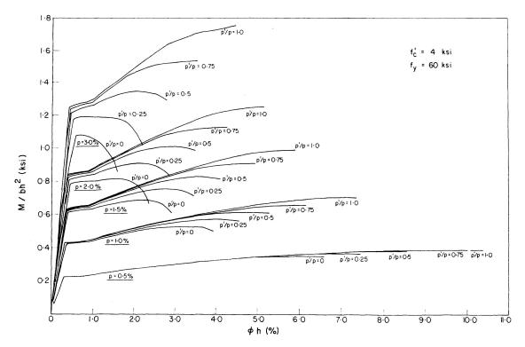
Fig. 12. Effect of compression reinforcement on ductility: M- $\phi$  diagrams.
