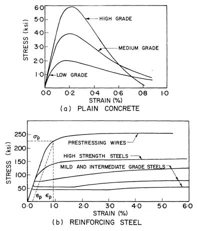
Fig. 1. Typical stress-strain curves for (a) concrete in compression and (b) reinforcing steel.
