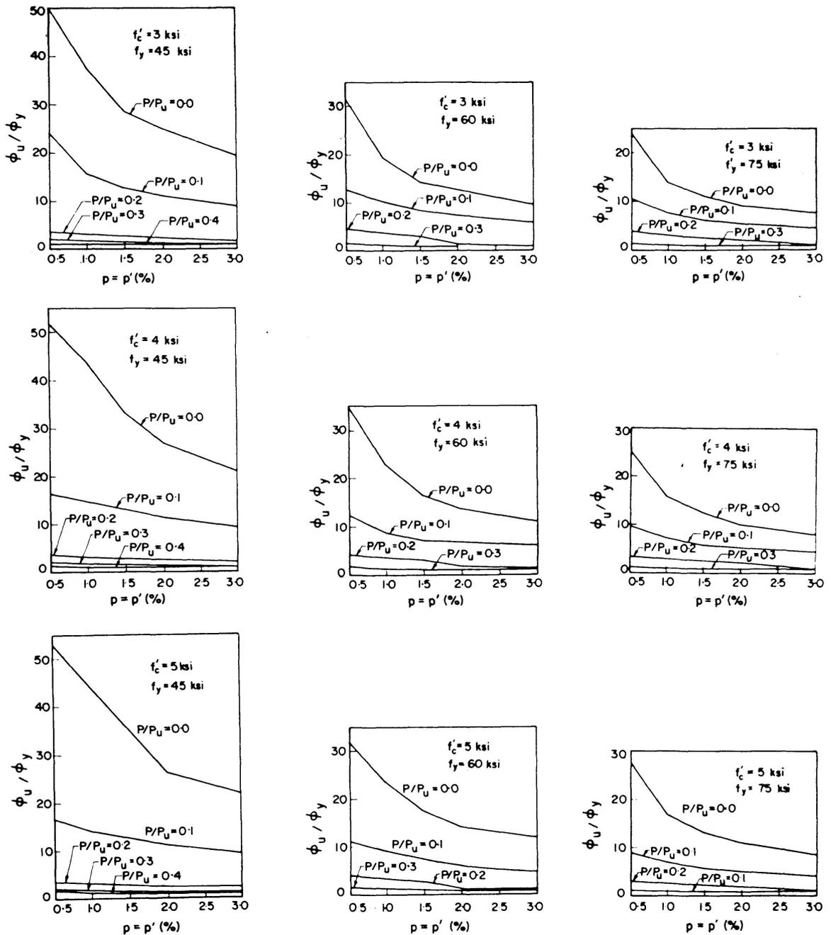
Fig. 23. Effect of axial loads on ductility:  $\phi_u/\phi_y$ - $p$  diagrams.
