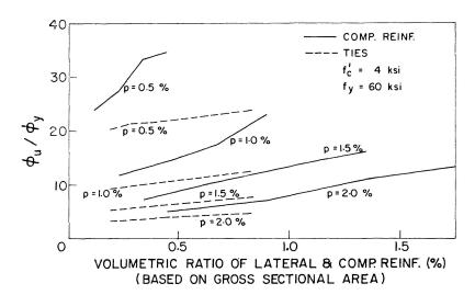
Fig. 17. Relative effect of compression and lateral reinforcements on ductility.
