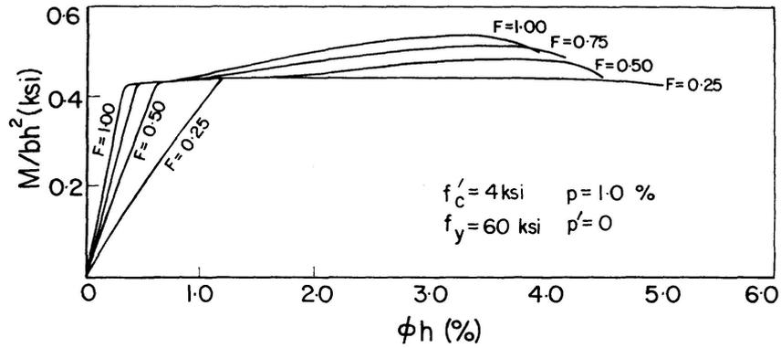
Fig. 8. Effect of bond on ductility:  $M-\phi$  diagrams.
