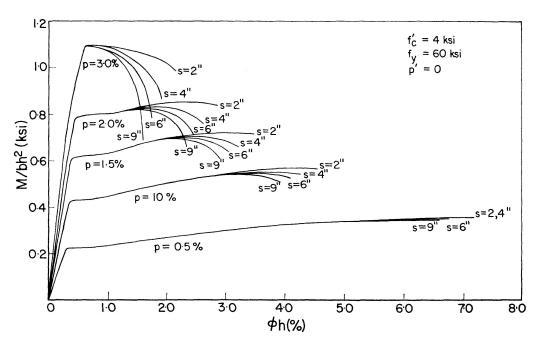
Fig. 14. Effect of tie spacing on ductility:  $M-\phi$  diagrams.
