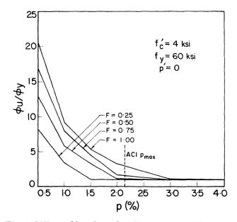
Fig. 9. Effect of bond on ductility:  $\phi_u/\phi_y$ -p diagrams.
