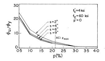
Fig. 15. Effect of tie spacing on duetility:  $\phi_u/\phi_y$ -p diagrams.
