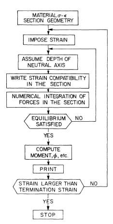
Fig. 3. Flow diagram for numerical analysis.
