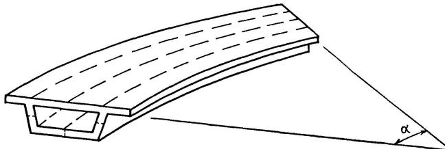
Fig. 1a. A Curved Box Bridge and It's Idealization into Strips.
