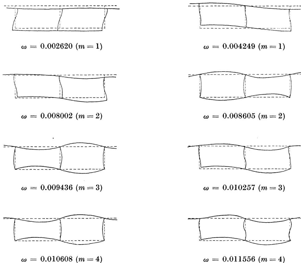
Fig. 3. Modal Shapes of a Curved Box Girder Bridge ( $E = 1$ ,  $\nu = 0.16$ ,  $\rho = 1$ ).
