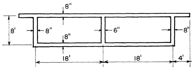
Fig. 2c. Section of the Box Girder Bridges.
