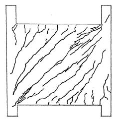
Experimental Crack Pattern from Ref. 2, Vol. 2, p. 128.
