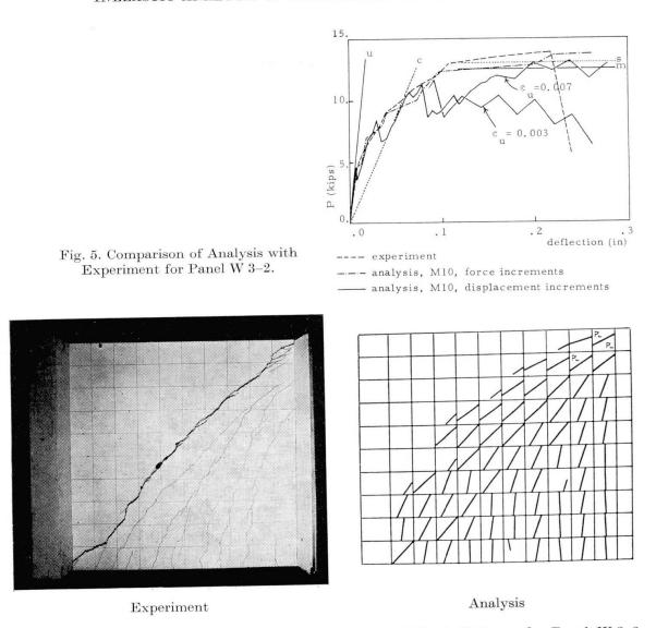
Fig. 6. Comparison of Final Analytical and Experimental Crack Patterns for Panel W 3-2.
