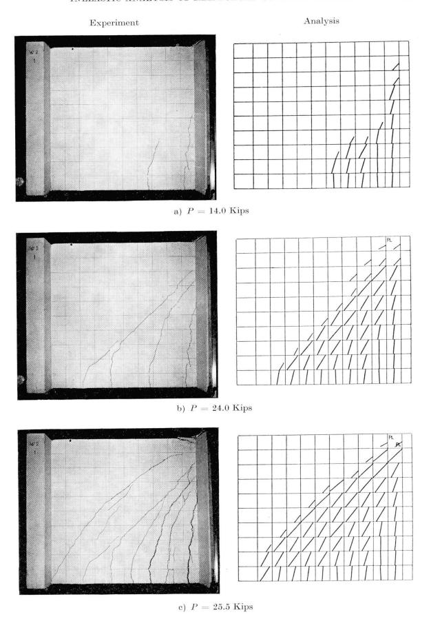
Fig. 4. Comparison of Analytical and Experimental Crack Patterns for Panel W 2.
