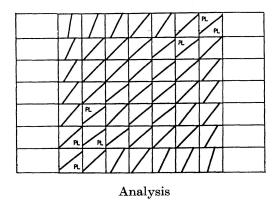
Fig. 12. Comparison of Analytical and Experimental Crack Patterns at Failure for Beam 391.
