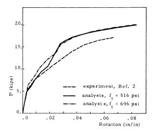
Fig. 11. Comparison of Analysis with Experiment for Beam 391.
