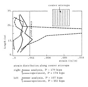
Fig. 14. Comparison of Analytical and Experimental Strains in Vertical Reinforcement.
