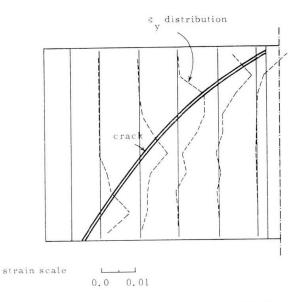
Fig. 7. Panel W 3-2. Diagonal Crack Location from the Distribution of Anlytical Strains  $\epsilon_y$ .
