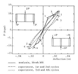
Fig. 8. Comparison of Analysis with Experiment for Specimen W 4 under Elastic Cycling.
