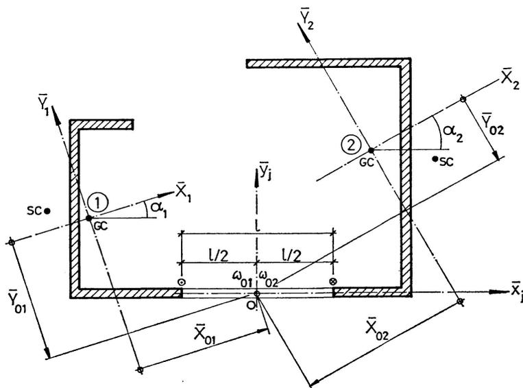
Fig. 3. Cross section of coupled nonprismatic shear wall.
