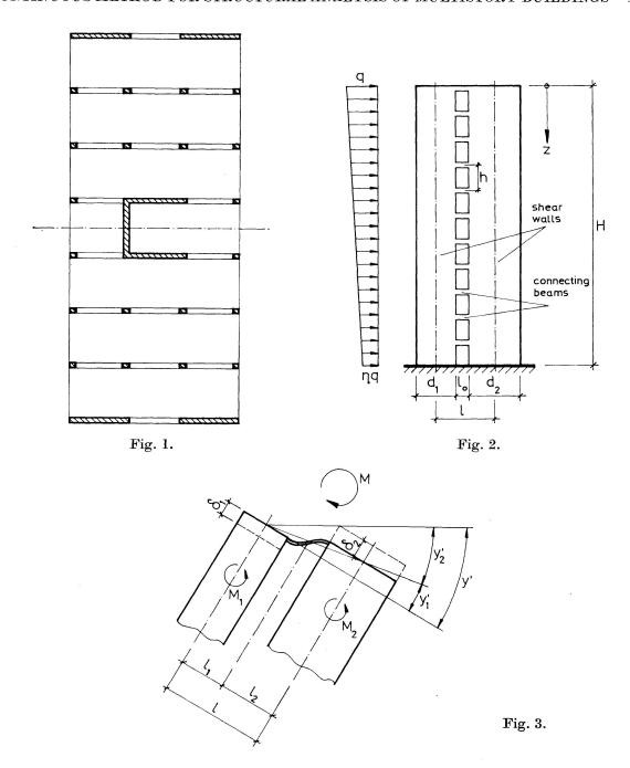
in which  $M_i$  = moment in the shear wall "i"; N = normal force in the shear wall due to lateral loads; and l = distance between shear wall center lines (see Fig. 2).
