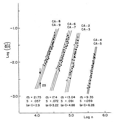
Fig. 6. Strain Accumulation per Cycle vs. Equivalent Number of Cycles.
