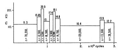
Fig. 9. Variable Amplitude Multi-Step Test 5.
