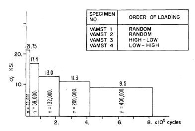
Fig. 8. Variable Amplitude Multi-Step Tests 1-4.
