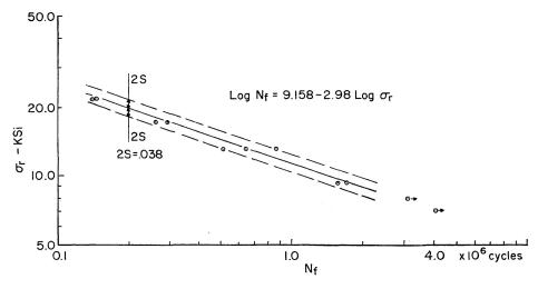
Fig. 5. Stress Range vs. Cycles to Failure.
