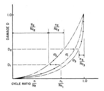
Fig. 3. Damage Accumulation due to Variable Amplitude Loads.
