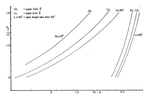
Fig. 13.  $N_f$ ,  $\alpha$  Curves for 2 S-1 Truck Type.
