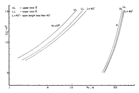
Fig. 11.  $N_f$ ,  $\alpha$  Curves for 2 D Truck Type.
