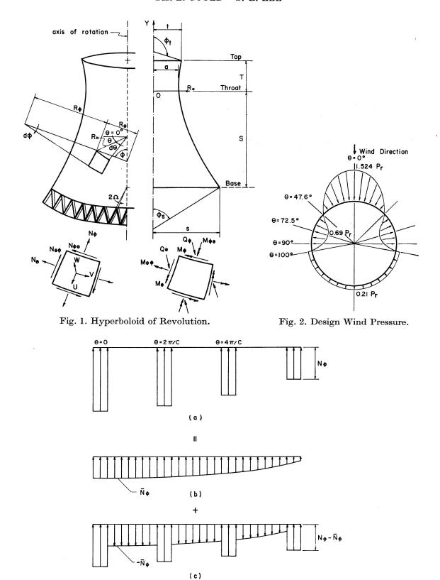
Fig. 3. Superposition Representation of Column Reactions.
