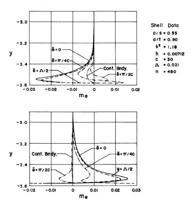
Fig. 5. Bending Stress Resultants – Circumferential Variation  $\theta=0^{\circ}$ .
