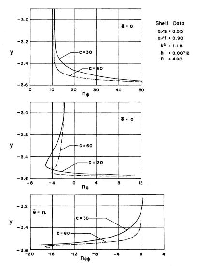
Fig. 7. Membrane Stress Resultants – Effect of Column Spacing  $\theta = 0^{\circ}$ .
