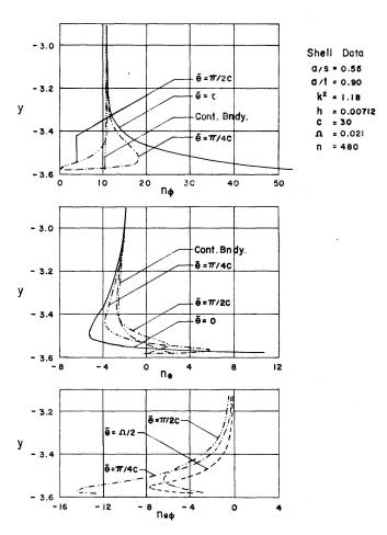
Fig. 4. Membrane Stress Resultants – Circumferential Variation  $\theta = 0^{\circ}$ .
