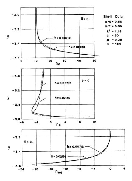
Fig. 9. Membrane Stress Resultants – Effect of Shell Thickness  $\theta = 0^{\circ}$ .
