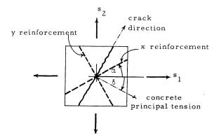
Fig. 8. Deviation of Crack Direction from Total Principal Stress Direction Caused by Reinforcement.
