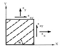
Fig. 5. Total Stresses  $\{s\}$  in the element of Reinforced Concrete Panel.
