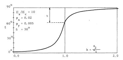
Fig. 9. Effect of Stress State on the Deviation of Concrete Principal Directions.
