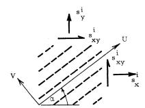
Fig. 7. Reinforcement Stresses  $\{s^i\}$ .
