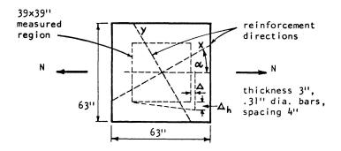
Fig. 10. Peter's Test Panel Subjected to Uniaxial Tension.
