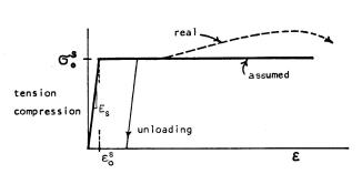
Fig. 4. Uniaxial Stress-Strain Relation for Steel Reinforcement.
