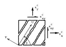
Fig. 6. Concrete Stresses  $\{s^c\}$  in the Cracked Concrete.
