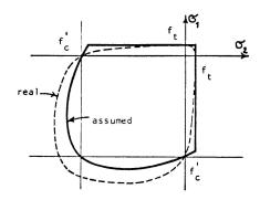
Fig. 3. Biaxial Strength of Concrete.
