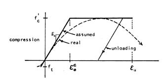
Fig. 2. Uniaxial Stress-Strain Relation for Concrete.
