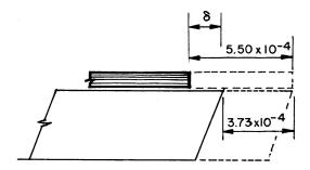
Fig. 6. Strain Movements at End of Member.
