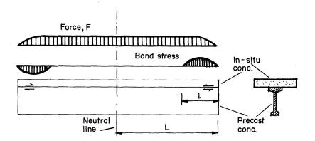
Fig. 1. Interface Force Between Two Concretes.
