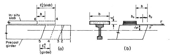
Fig. 5. Strain Movement of Concretes and Differential Shrinkage.
