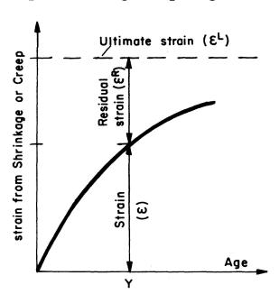
Fig. 4. Strain vs. Age of Concrete Due to Shrinkage or Creep Under Stress (Typical Diagram).
