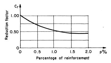
Fig. 3. Reduction Factor for Restraint in Strain vs. Percentage of Steel.
