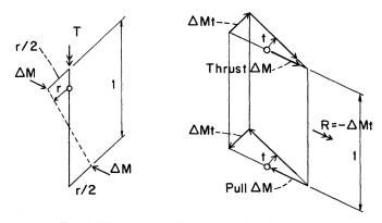
Fig. 6. Response of moment load on arch.
