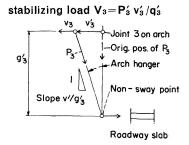
Fig. 5. Changing direction of buckling loads.
