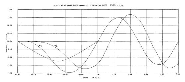
Fig. 6. Plate response to moving force.
