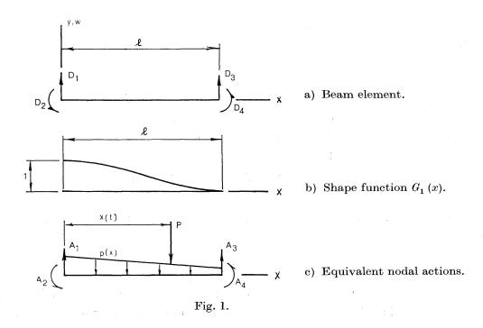
Shape functions assumed for the four types of nodal displacements of this element are:
