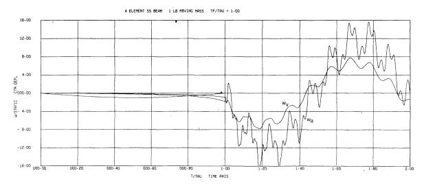
Fig. 7. Beam response to moving mass.
