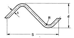
Fig. 11. Cross-Section of Corrugation.
