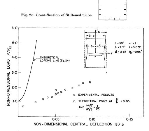
Fig. 26. Load-Deflexion Behaviour of Stiffened Plate.
