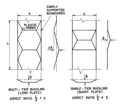
Fig. 4. Plastic Mechanisms.
