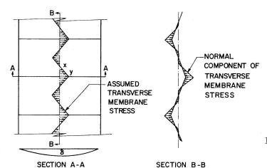
Fig. 5. Mechanism for Long Stiffened Plate.
