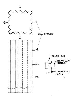
Fig. 9. Tube with Corrugated Walls.
