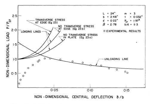
Fig. 14. Load-Deflexion Behaviour of the Corrugated Plate (Type II).
