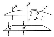
Fig. 8. Moment Distribution Across the Stiffened Plate.
