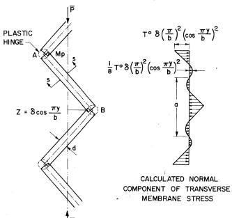
Fig. 6. Buckled Shape and Membrane Action in Corrugated Strip.
