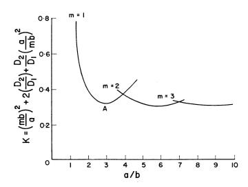
Fig. 2. Buckling Coefficients for Simply Supported Stiffened Plate.
