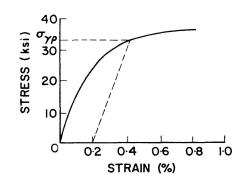
Fig. 10. Stress-Strain Relationship 575-H 34 Aluminum Alloy.
