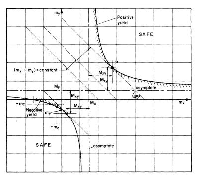
Fig. 1. The yield curve for orthogonal reinforcement.
