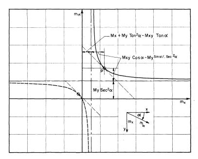
Fig. 6. The yield curve for skew reinforcement.
