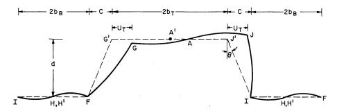
Fig. 3. Portal Frame Deformations at End of Panel.
