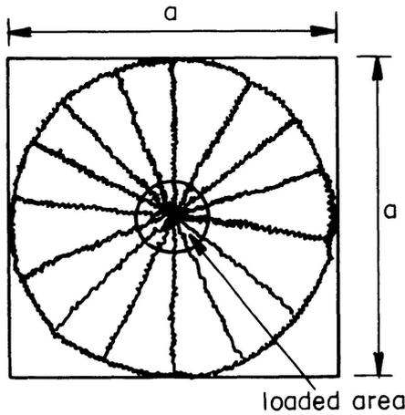
Fig. 2. Yield line pattern for case I - (Slab does crack beneath load).
