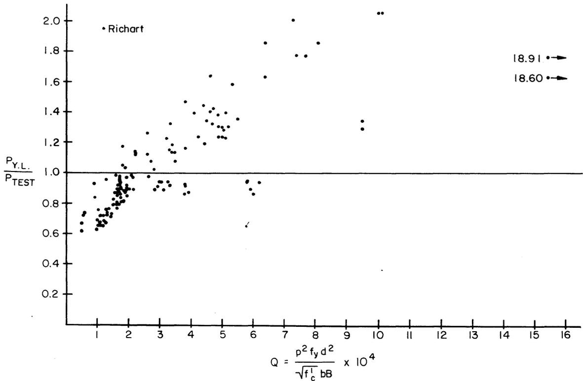
Fig. 9. Yield line load / Test load.
