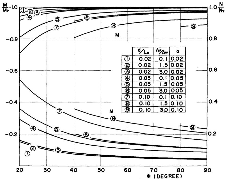
Fig. 16. Critical Bending Moment and Axial Thrust at Hinge "b" Under Combined Loading.
