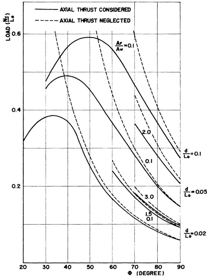
Fig. 11. Ultimate Load (Uniform Loading).
