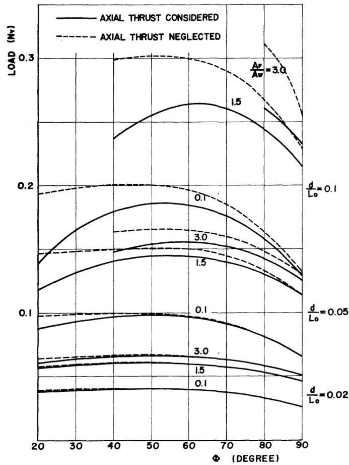
Fig. 12. Ultimate Load (Combined Loading).
