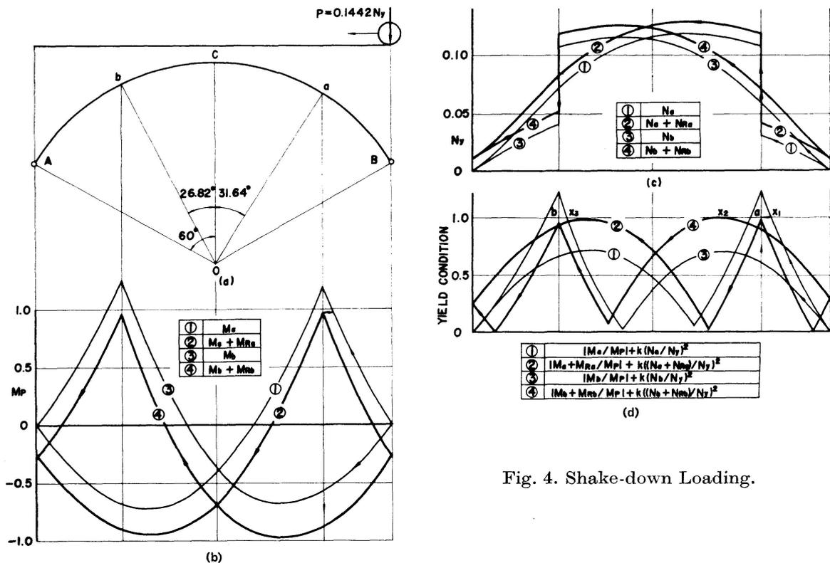
Fig. 4. Shake-down Loading.
