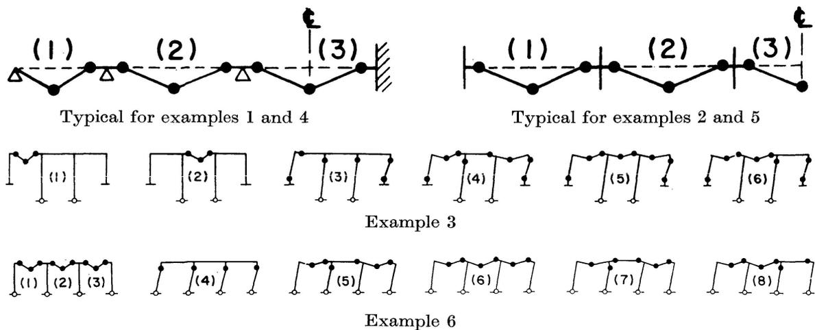
Fig. 3. Collapse modes of example structures.
