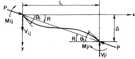
Fig. 2. Notations for the slope deflection equation.
