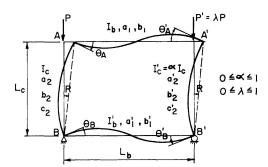
Fig. 3. Unsymmetrical frame unsymmetrically loaded.
