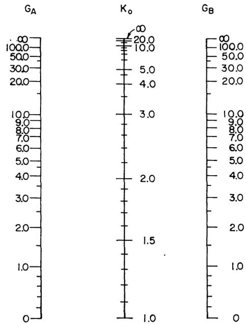
Fig. 6. Chart for the determination of  $K_0$ . (After AISC Manual of Steel Construction.)
