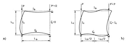
Fig. 4. Comparison of the deflection pattern of the case P'=0 and  $I'_c=0$  with the symmetrical case.
