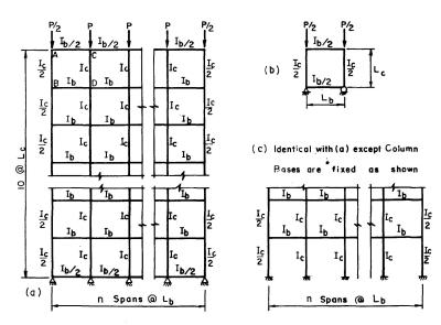
Fig. 7. (a) Frame solved in example 1. (b) A unit of the frame shown in (a). (c) Frame solved in Bleich's book.
