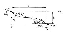
Fig. 2. Notations for the slope deflection equation.
