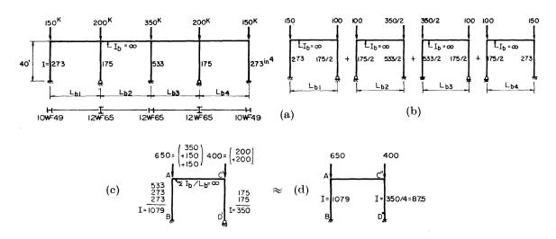
Fig. 11. (a) Frame solved in example 5. (b) Superposition of frames. (c) An equivalent frame. (d) Final equivalent frame.
