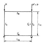
Fig. 1. Symmetrical frame symmetrically loaded.
