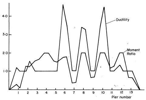
Fig. 9. Ductility required in deck beam.
