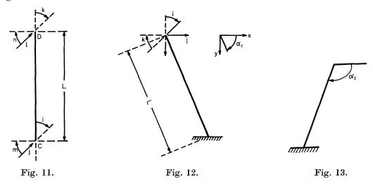
With the inclined members it is only necessary to consider the equilibrium of one joint as the other end is fully fixed. For a pier member inclined at angle  $\alpha$  to the horizontal x axis (see fig. 12), there are three unknown deformations and the member equilibrium equations may be written:
