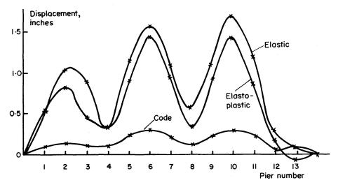
Fig. 7. Response of deck beam.
