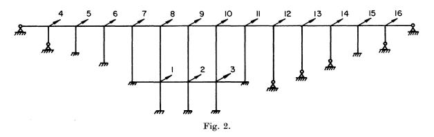
of the structure. There were also two rotations associated with each lateral displacement, one about the vertical pier axis and one about the deck beam axis. This means that when the equations of equilibrium for the structure are written it is necessary to consider the torsional stiffness of the beam and column members.
