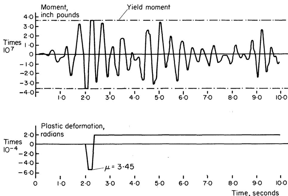
Fig. 8. Moment in deck beam between piers 9 and 10.
