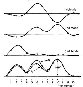
Fig. 3. Curve A: Predicted elastic response by R.M.S. Curve B: Response by direct integration.
