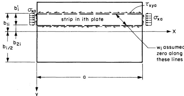
Fig. 2. Strip element of typical ( $i$ th) plate.
