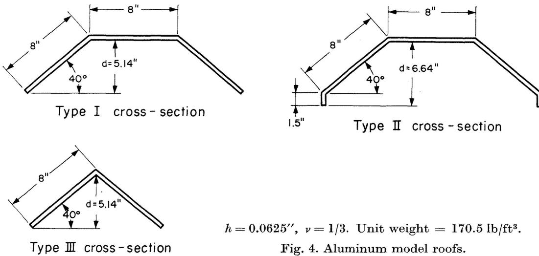
and longitudinal stresses for span to depth ratios less than about eight to one. For larger ratios the center plates buckled under the action of longitudinal stresses. The Type III roofs buckled under a combination of shearing and longitudinal stresses. The optimum number of strips for inclined plate buckling was two and for the center plate buckling was one.
