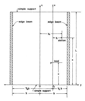
Fig. 1. Coordinate axes for point load acting on bridge deck.
