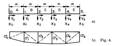
The stress diagram in the plate is assumed to have a polygonal form. Each intermediate nodal concentration, normal or tangential, is converted into a triangular area with the base 2m of the stress diagram directly underneath the node. Thus, with the thickness of the plate t,
