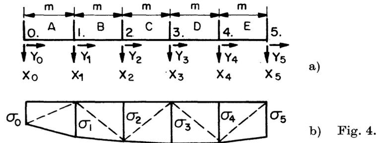
The stress diagram in the plate is assumed to have a polygonal form. Each intermediate nodal concentration, normal or tangential, is converted into a triangular area with the base  $2m$  of the stress diagram directly underneath the node. Thus, with the thickness of the plate  $t$ ,
