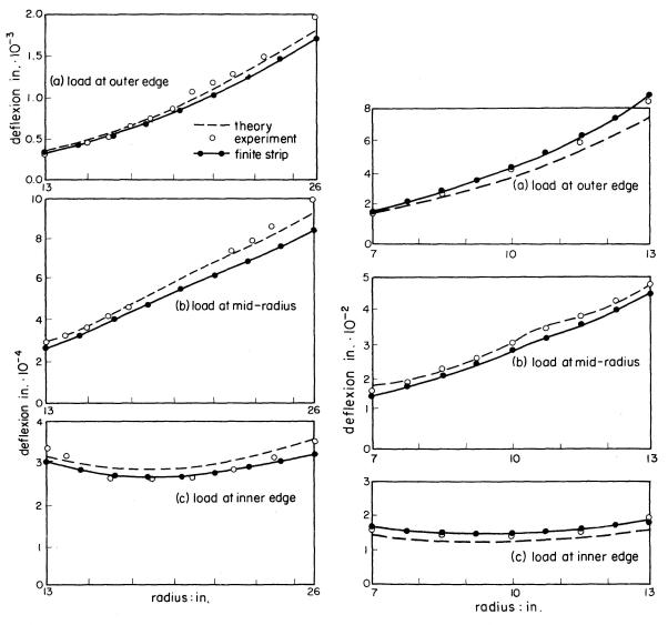
Fig. 2. Radial distributions of mid-span deflexions due to unit load at (a) outer edge, (b) mid-radius, (c) inner edge; asbestoscement model.
