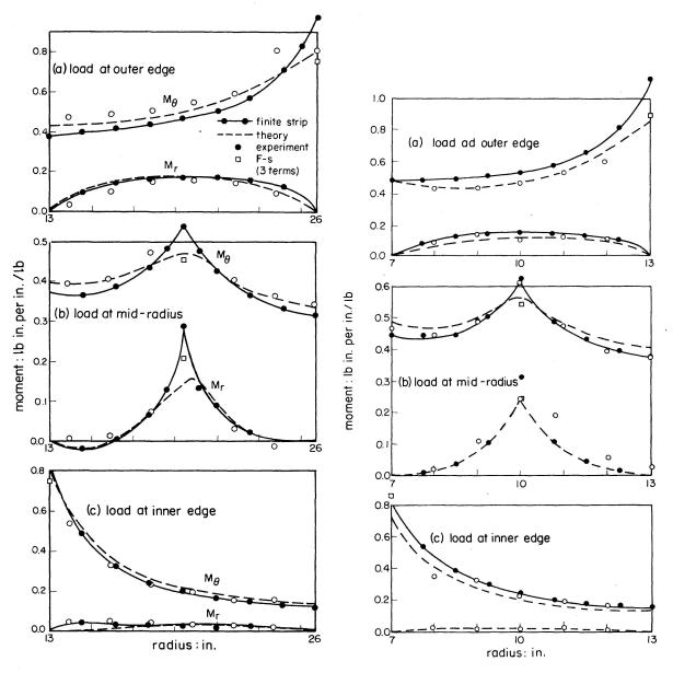
Fig. 4. Distributions of tangential and radial bending moments at mid-span due to load at (a) outer edge, (b) mid-radius, (c) inner edge; asbestos-cement model.
