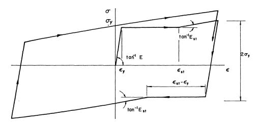
Fig. 13. Stress-strain diagram.
