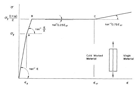
Fig. 16. Tension specimen model.
