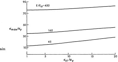
Fig. 10. Maximum strain  $(P/P_p = 1.0)$ .
