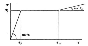
Fig. 1. Stress-strain diagram.
