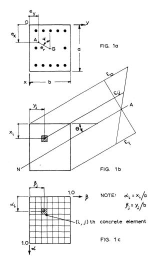
Fig. 1. Cross section details.
