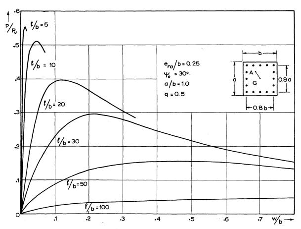
Fig. 5. Load deflection curves; various column lengths.
