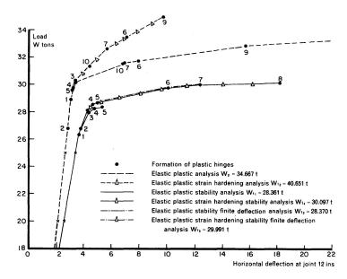
Fig. 6. Elastic plastic strain hardening load deflection curves for Wood's frame. Steel to B.S. 968: 1962.
