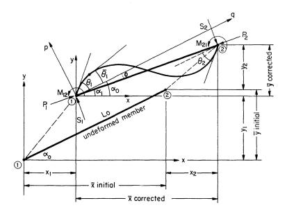
Fig. 1. The deformed member.
