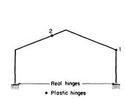
Fig. 9. Order of hinge formation for the B.C.S.A. portal frame. Steel to B.S. 968: 1962. All members
