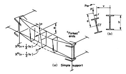
Fig. 8. Lateral buckling.
