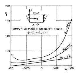
Fig. 3. Middle surface direct longitudinal stress at the crest of a buckle.
