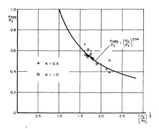
Fig. 8. Maximum strength of eccentrically loaded short lipped channel struts.
