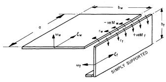
Fig. 4. Geometry and edge restraint representation of component plates of a lipped channel.
