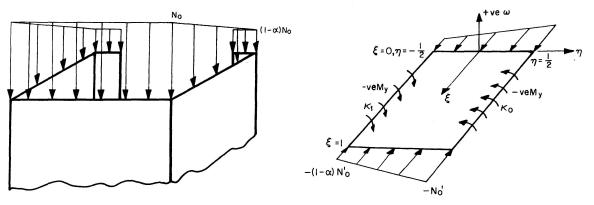
Fig. 1. Channel loading geometry.
