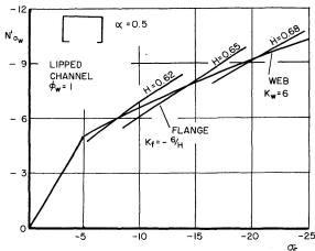
Fig. 5. Variation of load with longitudinal direct stress at  $\eta = \frac{1}{2}$ .
