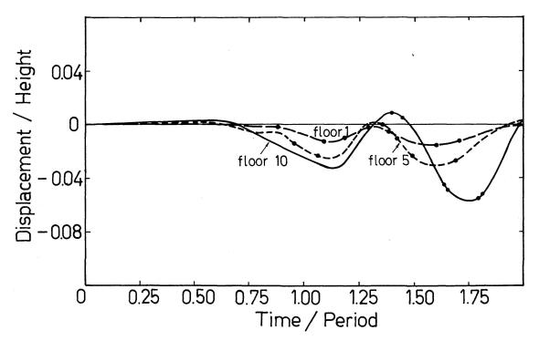
Fig. 1. Deflection response curves for floors 1, 5 an 10 ( $\alpha = 0.10$ ).
