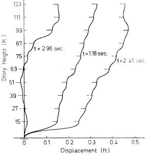
Fig. 6. Deflected position of 10-story column at selected times ( $\alpha = 0.10$ ).
