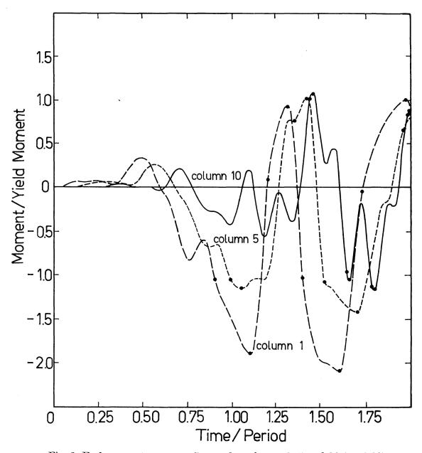
Fig. 2. End moment response Curves for columns 1, 5 and 10 ( $\alpha = 0.10$ ).
