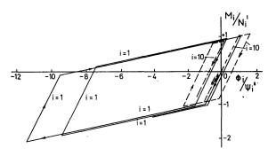
Fig. 5. End moment-curvature history of columns 1 and 10 for  $\alpha = 0.1$ ,
