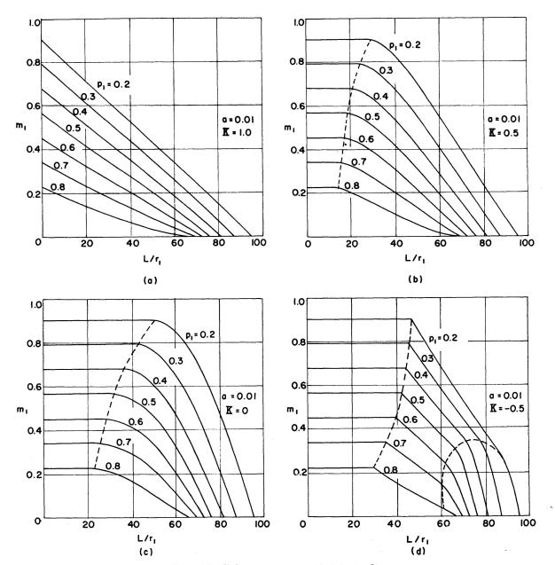
Fig. 13. Column curves (A 36 steel).
