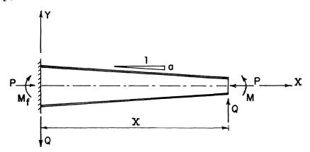
Fig. 2. Tapered wide-flange cantilever column under arbitrary end loads.
