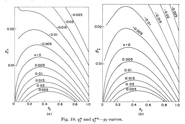
The intersection of the upper and lower envelopes is the same as the common point  $(x^*, m^*)$  of the elastic equilibrium curves as long as  $q_f \le q_f^*$ . When  $q_f$  exceeds  $q^*$ , neither the elastic equilibrium curve nor the common point exists. However, the numerical value of  $m^*$  can still be computed as if the column were infinitely elastic. For  $q_f^* < q_f \le q_f^{**}$ , it can be shown that the point  $(x^*, m^*)$  still defines the intersection of the envelopes.
