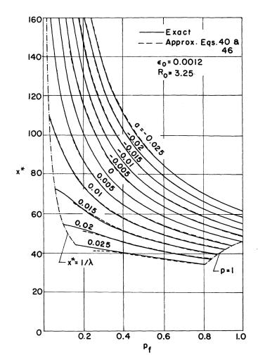
Fig. 6. Euler lengths of tapered cantilever columns.
