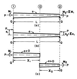
Fig. 11. Simply supported tapered columns.
