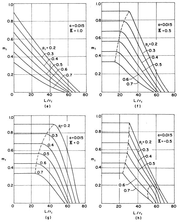
Fig. 13. Column curves (A 36 steel).
