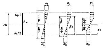
Fig. 3. Cross section and stress distribution due to bending and compression.
