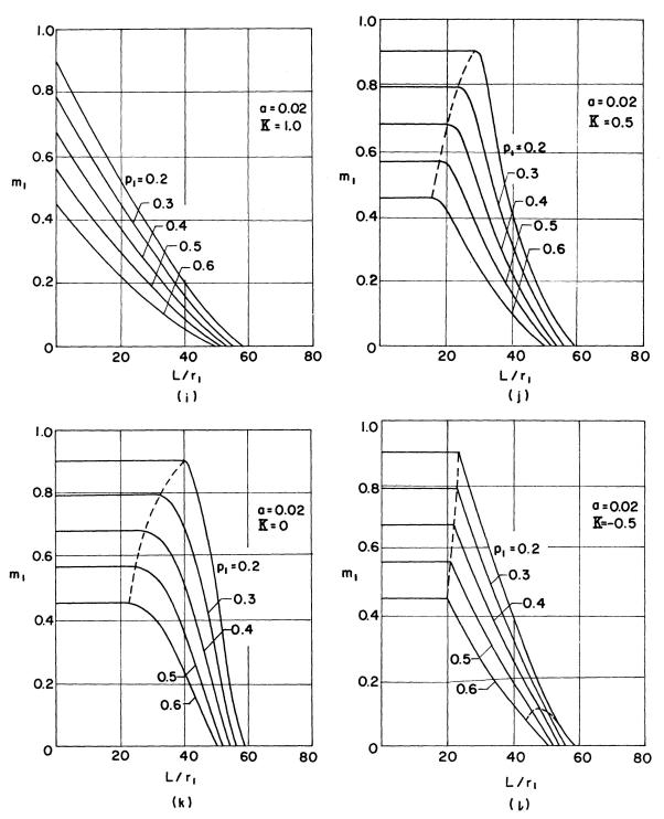
Fig. 13. Column curves (A 36 steel).
