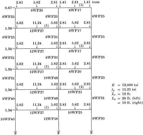
Note: Frame 6—1 shown. Frame 6—2 is identical except for half vertical loads in girder spans marked [1].
