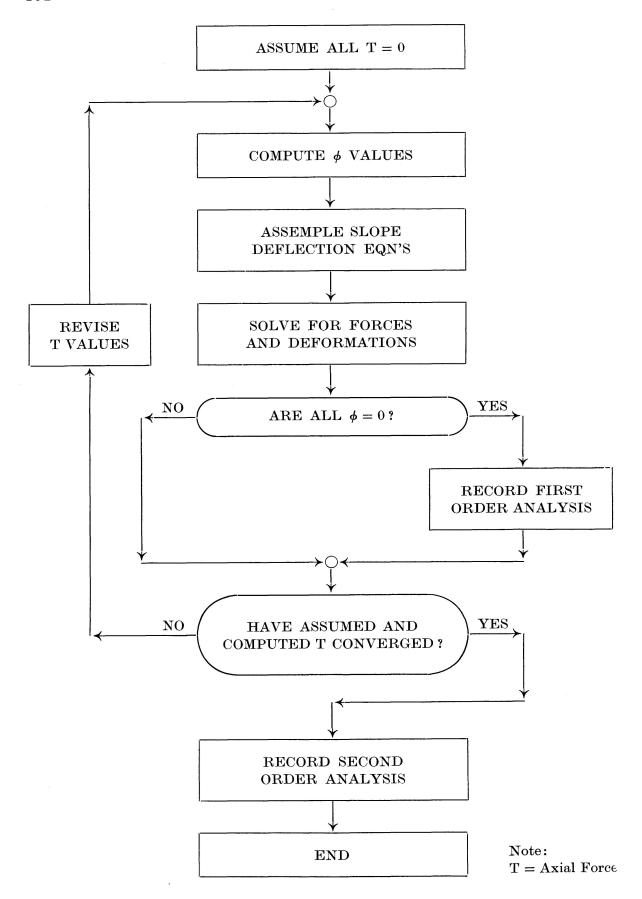
Fig. 2. Flow chart; unified elastic analysis.
