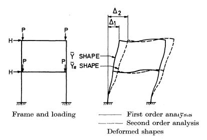
Fig. 1. Elastic frame deformations.
