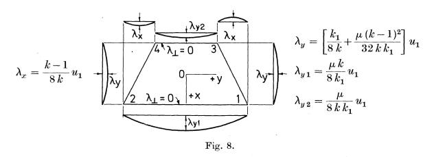
Edge 1—2. The normal displacements are linear. The nodes 1 and 2 move to the left (Fig. 5) the amount  $\frac{\mu \, k}{2 \, k_1} \varDelta_D = \frac{\mu \, k}{8 \, k_1} \, u_1$ , while the mid-point remains at rest. The relative tangential displacement of the midpoint in relation to the ends is  $\lambda_{y\,1} = + \frac{\mu \, k}{8 \, k_1} \, u_1$ .
