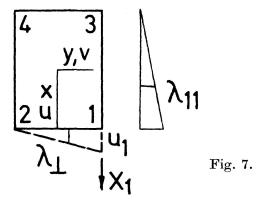
that of all edge displacements only  $\lambda_1$  on the edge 1—2 and  $\lambda_{11}$  on the edge 1—3 are distinct from zero. Employment of the influence lines of the type of  $\lambda_1$  and  $\lambda_{11}$  in Fig. 7 for calculation of  $X_1$  is obviously equivalent to the application of the law of the lever. Under the stated conditions the terms  $X_1$  found by the two methods should then be identical.
