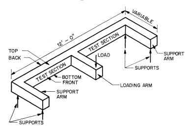
Fig. 1. Specimens and loading scheme.
