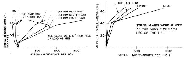
Fig. 4. Strain gage readings for specimen 2. Fig. 5. Strains in one tie of specimen 7.
