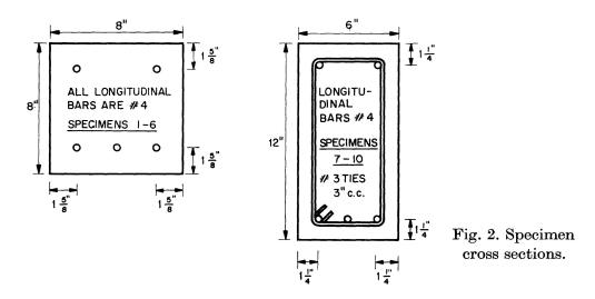
were tested between thirty and sixty days after being cast. The accompanying cylinders were tested at the same time as the specimens. Strengths are recorded in table I.
