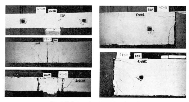
Fig. 6. Failure crack pattern of specimen 9.
