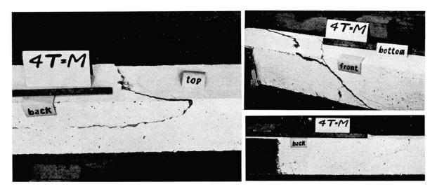
Fig. 3. Failure crack pattern of specimen 4.
