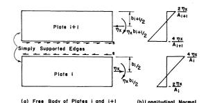
Fig. 2. Longitudinal normal stresses.
