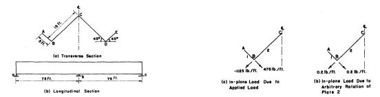
Fig. 4. Shell dimensions (example 1).
