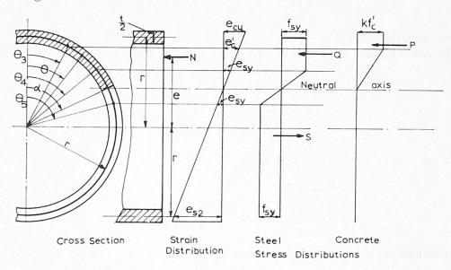
Fig. 2. Stress and strain distributions at ultimate load.
