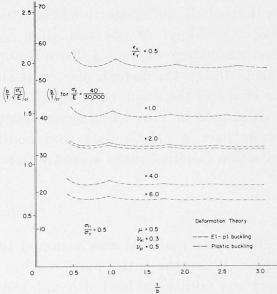
Fig. 15. Relationship between  $(b/t)_{cr}$  and (L/B) for  $\sigma_{r,1}/\sigma_{Y} = 0.5$ .
