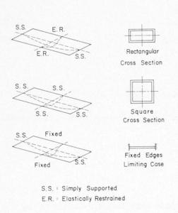
Fig. 5. Boundary conditions of the plates.
