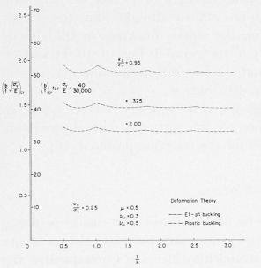
Fig. 14. Relationship between  $(b/t)_{cr}$  and (L/B) for  $\sigma_{r\,1}/\sigma_{Y}=0.25$ .
