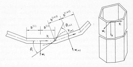
Fig. 4. Coordinate axes for plate elements.
