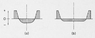
Fig. 1. Usual residual stress distributions in edge welded plates.
