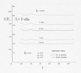
Fig. 13. Relationship between  $(b/t)_{cr}$  and (L/B) for  $\sigma_{r1}/\sigma_Y = 0.125$ .
