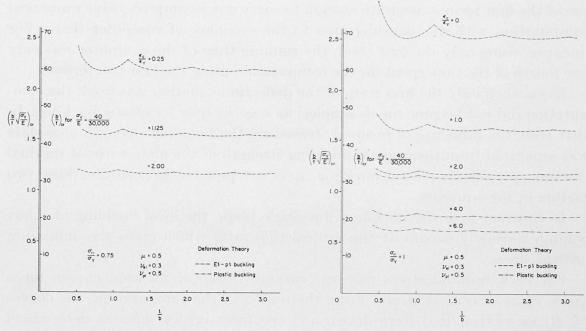
Fig. 16. Relationship between  $(b/t)_{cr}$  and (L/B) for  $\sigma_{r1}/\sigma_Y = 0.75$ .
