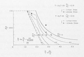
Fig. 19. Plate buckling curve with test points (A-514 steel).
