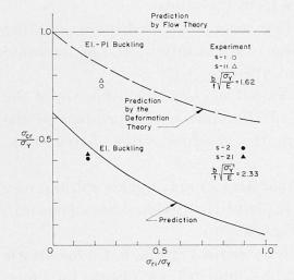
Fig. 20. Critical local buckling strength of columns (A 36 steel).
