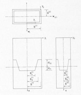
Fig. 6. Coordinate axes for a column of rectangular cross section.
